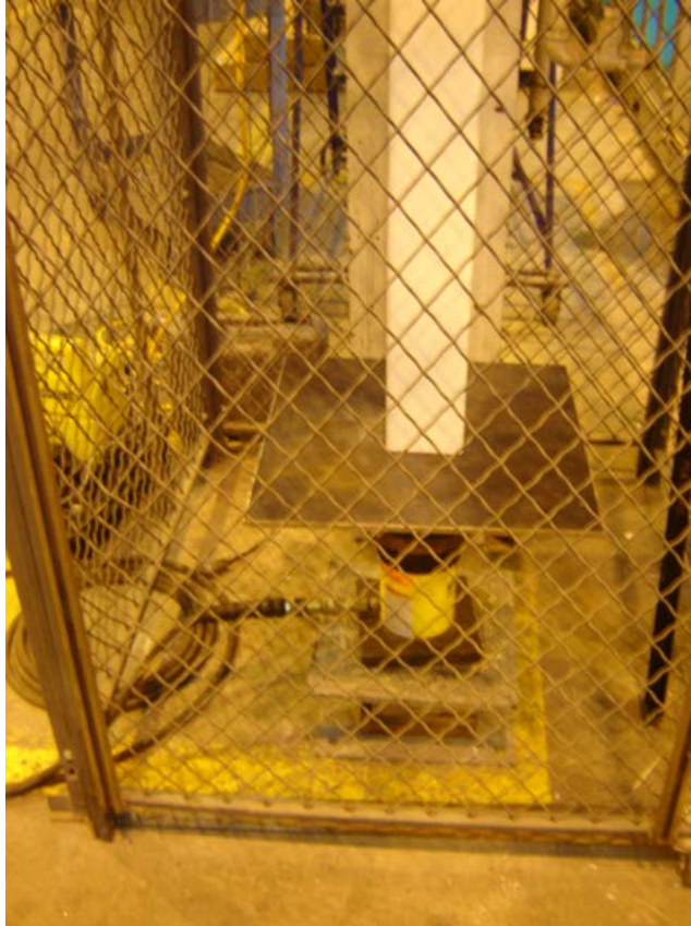
Photo No. 1 Column Base with Hydraulic Jack and Load Cell
