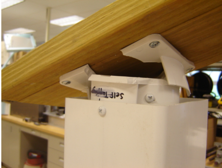
Photo No. 6 Uplift Load Test - Typical Mounting Bracket Fracture
