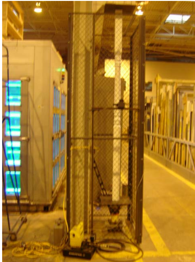
Photo No. 2 Axial Load Test Set-Up (4x4 Structural Porch Post)
