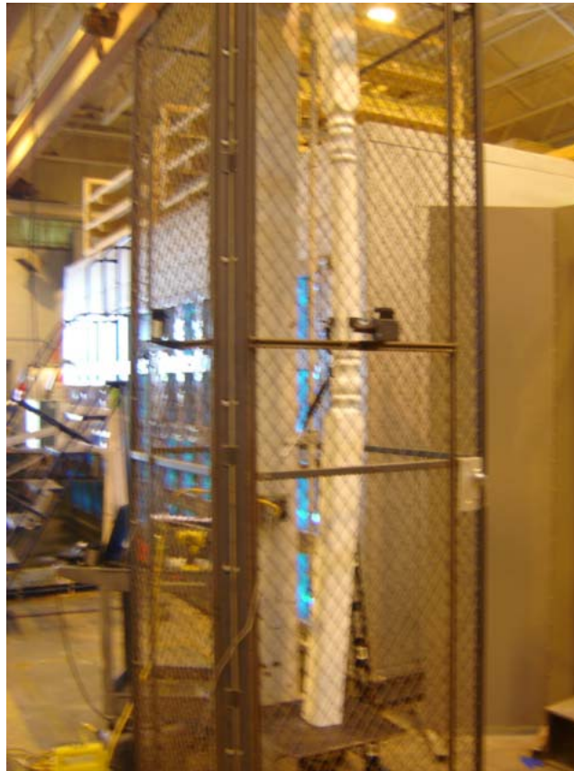
Photo No. 3 Axial Load Test Typical Buckling Failure of Specimen (4x4 Structural Porch Post)
